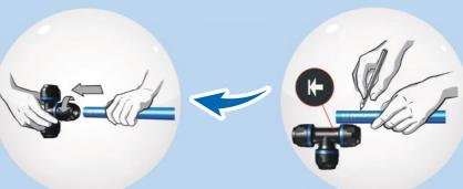
Unscrew the nut by several turns, and then insert the pipe while rotating it slightly until the recommended length is reached. NB: an assembly fluid (ref. PPS AL) is recommended to facilitate the assembly.
