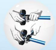
The pipe must be cut perpendicular to its length (ref. PPS CTU).
